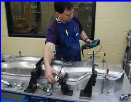
Die maker uses a DataMyte to input measurement data from a part on a check fixture.
