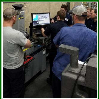
Employees received additional training on the "Zoller Tool Setter". This allows the CNC Machinist the ability to pre-measure tooling while the machine is running, reducing downtime and cost for the company.
