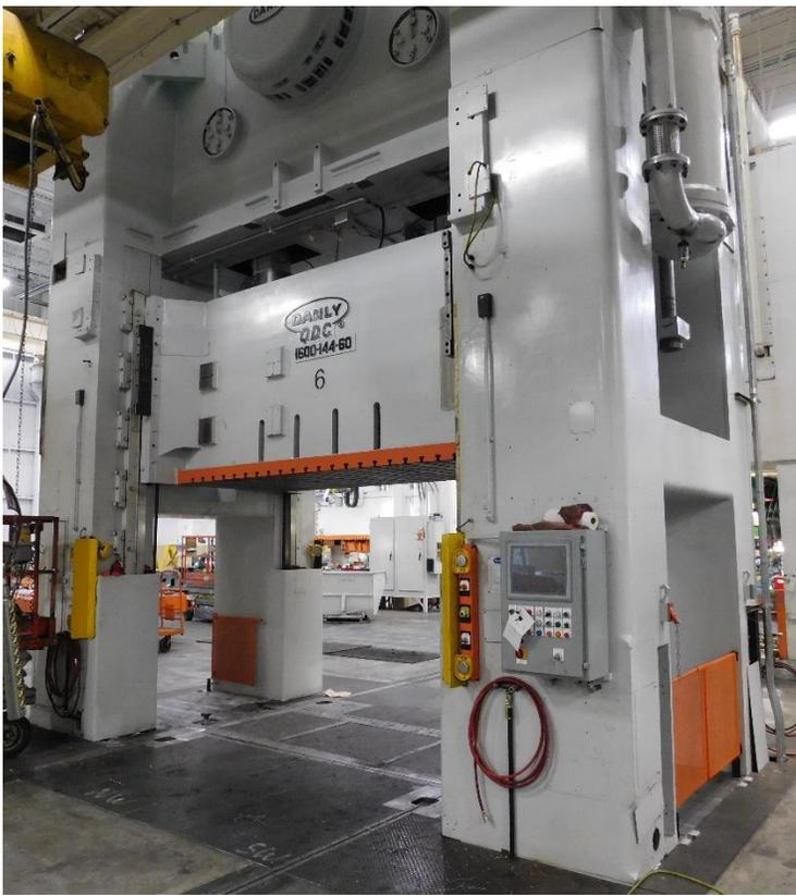
Greenville Tool & Die has installed this 1600 Ton Danly Press with a 30" stroke length, 18" slide adjustment, and capability of 9-18 strokes per minute. It is equipped with 72" x 144" rolling bolsters that maneuver both out the front and back.
